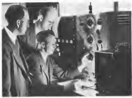
Propeller Parts Vibrated to Destruction: Ralph M. Gierke, chief experimental engineer of Curtiss-Wright Corp. Propeller Division, and one of his engineers, Charles Steffler and Ferret Dorman, checking a vibration test of the control panel of electronic apparatus in the experimental engineering laboratory. The laboratory is devoted to destruction in a short time propeller parts that would not fail in 10,000 hours of flight.
